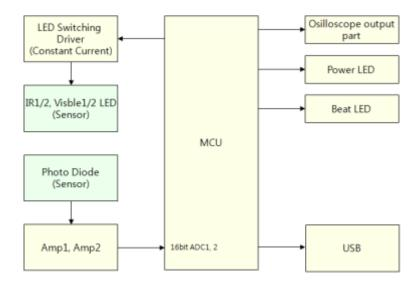
Measure the signals of each LEDs with the duty cycle 500Hz. The measured signals are amplified through Amp1 or Amp2. Amp1 is for IR1(905nm), IR2(810nm) and V1(660nm), Amp2 is for V2(570nm).
