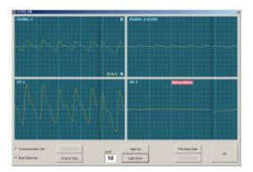
Left side is normal measuring case, Right low shows that IR2(801nm) was saturated.
