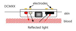
One of the major design considerations required in designing a reflectance pulse oximeter sensor is determining the optimum separation distance between the LEDs and the photodiode.
